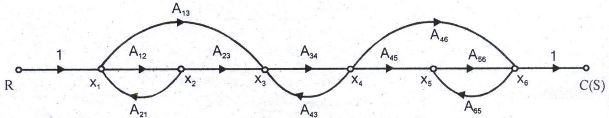
(ii) Using block diagram reduction technique, find the closed loop transfer function  $C/R$  of the system whose block diagram is shown in below (8)
